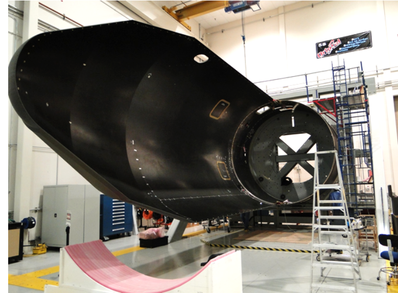
Test Stand with one 570-pound fairing loaded
